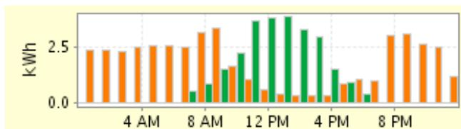
Size & shape of solar energy *made* (green) is predictably as before— roughly a parabola that matches (no surprise!) the sunshine and these are the hours usefully utilities charge most. PV production hasn't changed at all, since an EV was added to the equation.
