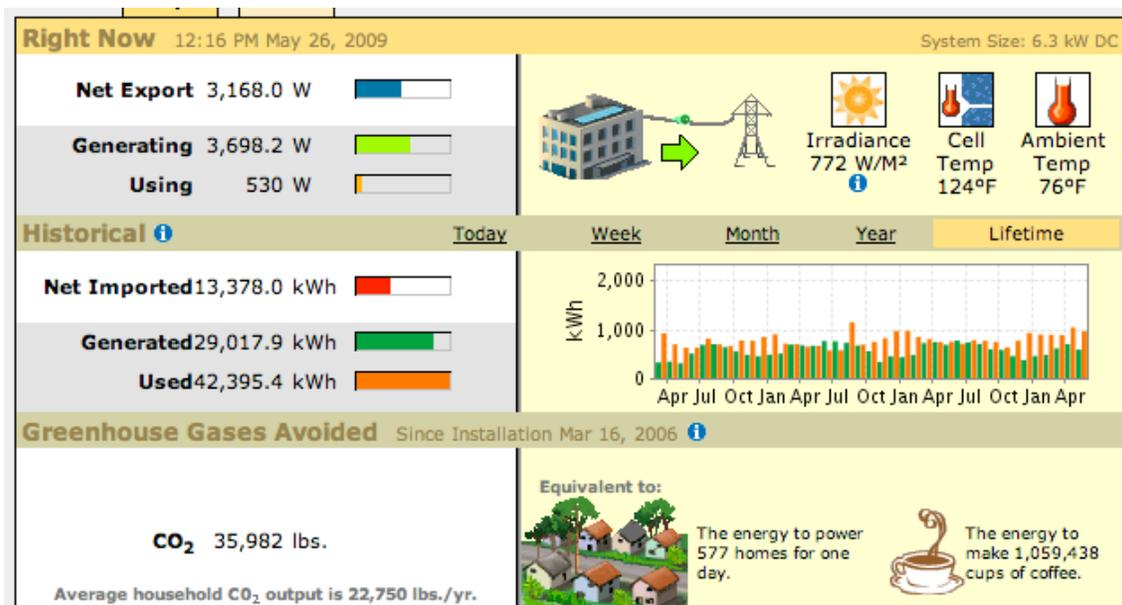
29,000 kWh was **generated** & measured since a 2<sup>nd</sup> PV monitoring was installed in 2006 (left). For this sample sunny On-peak moment (left, top), Irradiance is a sunny 772 W/M<sup>2</sup>; our PV is making 3,698 Watts, **demand** that moment is 530 Watts, and 3,167 Watts is being exported.
