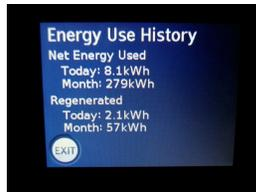
The EV used 279 kWh in May, or 350 after losses. Note 57 kWh of regen added range.
