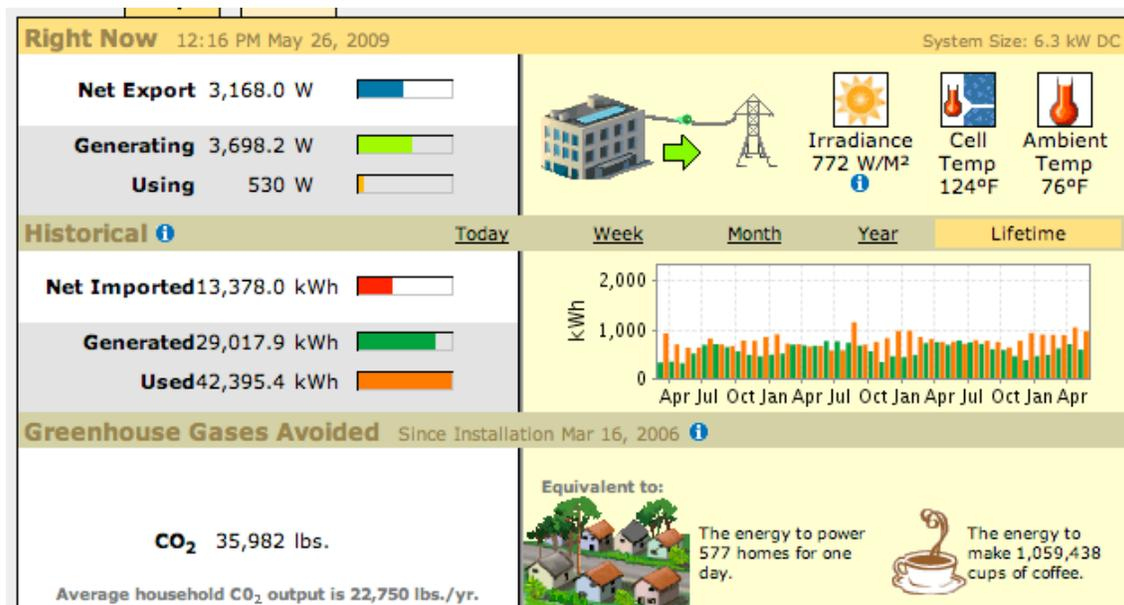
29,000 kWh was **generated** & measured since a 2<sup>nd</sup> PV monitoring was installed in 2006 (left). For this sample sunny On-peak moment (left, top), Irradiance is a sunny 772 W/M²; our PV is making 3,698 Watts, **demand** that moment is 530 Watts, and 3,167 Watts is being exported.
